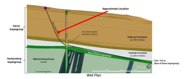
The next phase of drilling, planned for commencement this Saturday, will see the mobilisation of the Horizontal Directional Drilling rig, which will see a string of 1.5km long being drilled into the sandstone to intercept the gas bearing structures within the two primary target zones, the upper Vryheid Formation Sandstones and Dwyka Group Diamictite.
